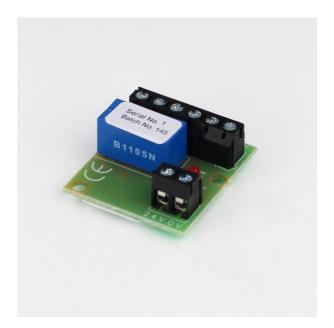
This is the miniature version of the IS 24. The 24 volt polarised double pole relay is a simple to fit module wherever a dry contact, voltage free switching is required. It is ideal for low current low voltage switching i.e. Industrial control systems and many other applications. The double pole relay is rated at 2 Amps complete with LED indication. It is supplied as an individual unit or in a strip of 4 modules.
